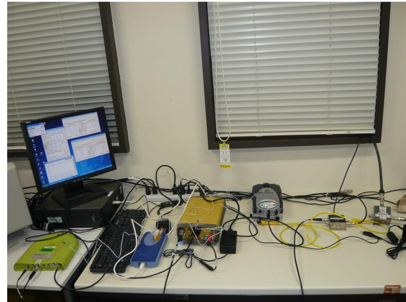
In the zero baseline, double-difference (DD) of code measurements can cancel out terms of orbital errors, clock errors, atmospheric delays and multipath, and remain DD of receiver noises and inter-channel biases.
