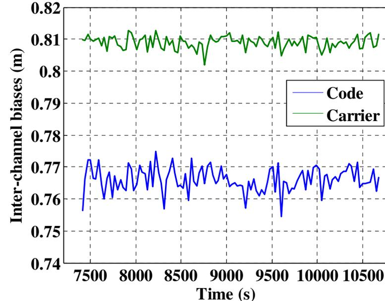
Inter-channel carrier bias can be obtained by subtracting the GLONASS integer ambiguity fixed in static mode from DD of carrier-phase measurement.
