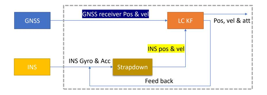
GNSS/INS loosely coupled means using GNSS position and velocity as Kalman filter measurements, which use it to estimate the INS. The Kalman filter will feed back the INS bias and output the position, velocity and attitude.
