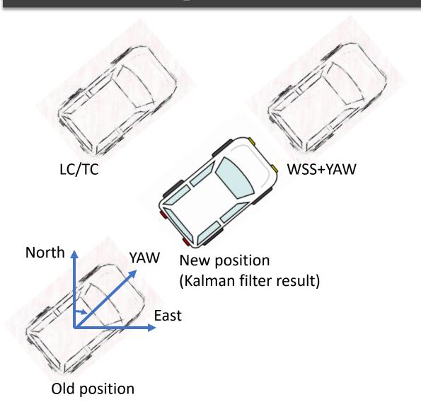
The WSS+YAW can provide the velocity in ENU. Using old position and velocity, we can get the WSS+YAW dead-reckoning position, do Kalman filter with the LC/TC position, can remove some error from the GNSS.
