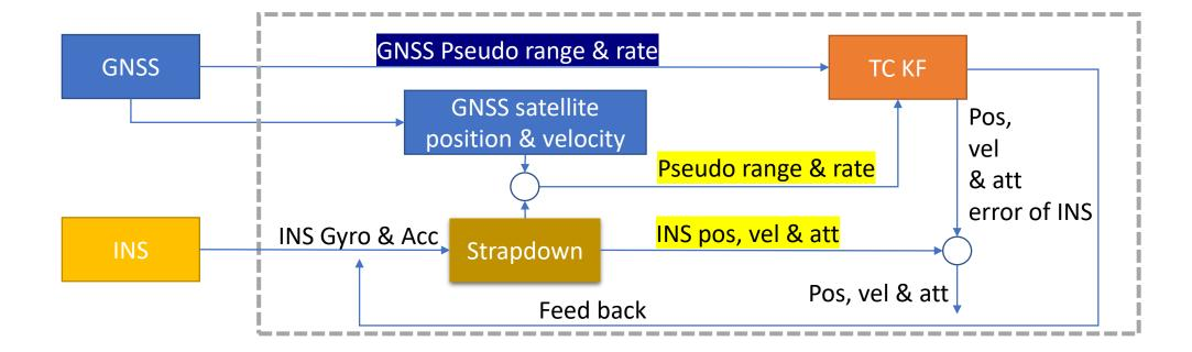
GNSS/INS tightly coupled means using GNSS pseudo range and pseudo range rate (Doppler frequency) as Kalman filter measurements, using INS position and velocity to calculate the estimate pseudo range and pseudo range rate, Kalman filter will estimate the INS errors, and eliminate the error of INS.
