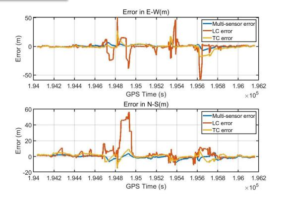
In the result of Marunouchi, the Multi-sensor fusion result is from the TC position and WSS+YAW. The maximum error is reduced, and positioning accuracy is improved.
