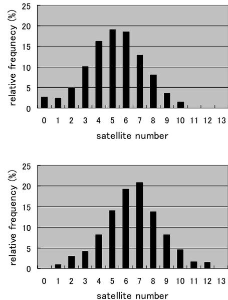
Figure 4. Relative frequency distribution (GPS and GPS+QZS)
