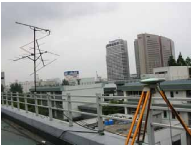
Photo 3 GPS Antenna Settled on the Roof of a Five-Storeyed Building at the Tokyo University of Marine Science and Technology
