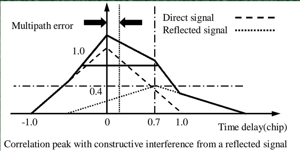
This picture shows correlation peak contaminated by a reflected signal. Most GPS receivers use a DLL (early-late correlator) to track the signal.
