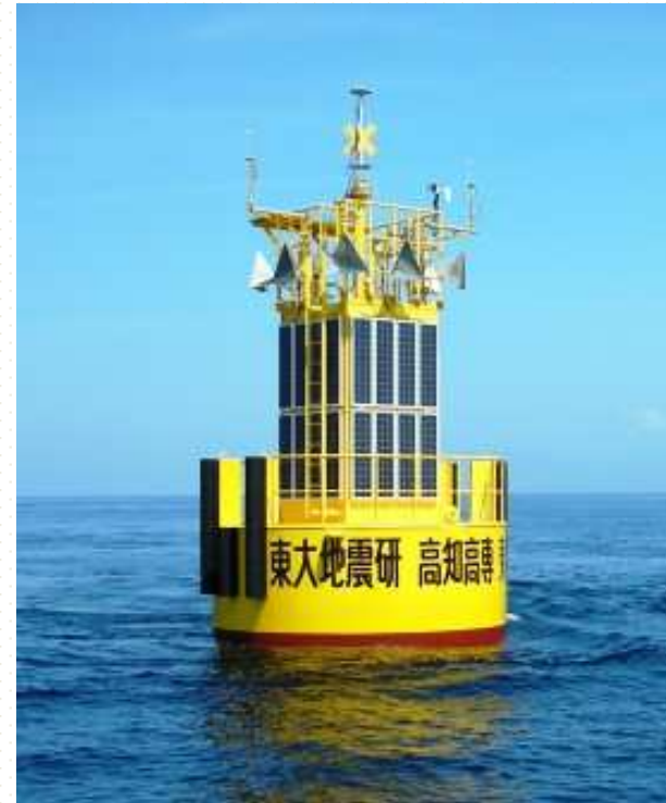
GPS Tsunami Monitoring System (Currently ~15 km off-shore)
